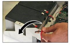
**4** Place the battery cables to the side and remove the used batteries.
